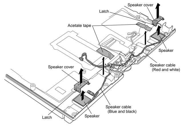
Figure 4-47 Removing the speaker
